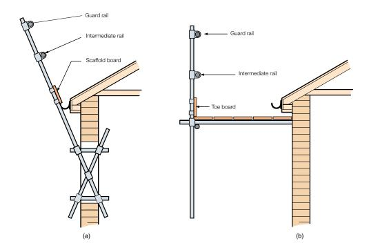
Figure 24 Example of flat-roof edge protection
