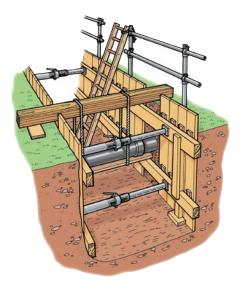
**Figure 44** An excavation supported by timbering and props with guard rails (omitted from left-hand side for clarity) to prevent falls. Extended poling boards act as toe boards, safe access is provided by a tied ladder and exposed services are supported
