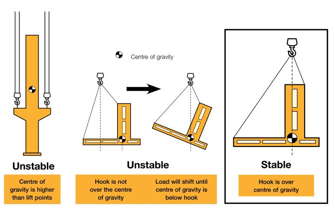
Figure 41 The centre of gravity must be beneath the hook
