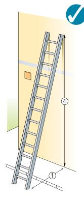
Figure 19 Ladder showing correct 1 in 4 angle (means of securing omitted for clarity)
