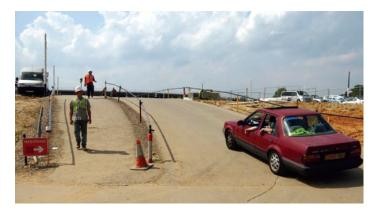
Figure 34 Pedestrians are segregated from vehicles on this slope
