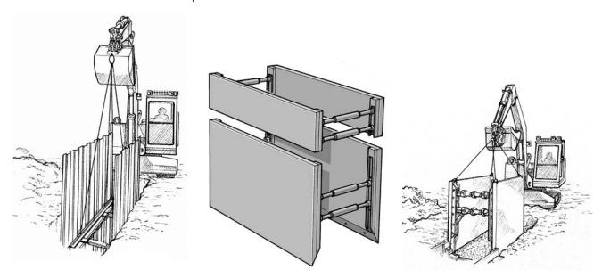
Figure 42 Proprietary trench boxes and hydraulic wallings allow trench supports to be put in place without requiring people to enter the excavation
