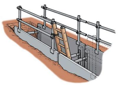
Figure 43 A trench box with guard rails attached
