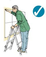
Figure 20a Correct – two clear rungs
