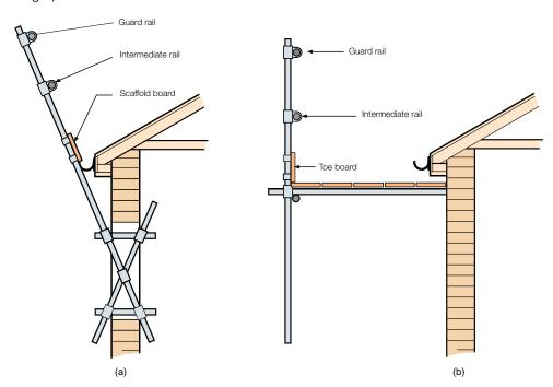
Figure 23 Typical sloping-roof edge protection
