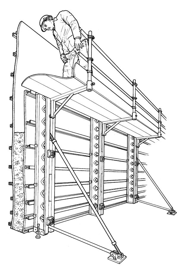
Figure 29 A formwork system with purpose-designed fittings
