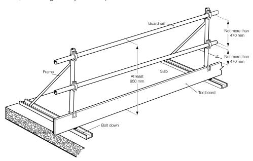
Figure 10 Guard rails and toe boards
