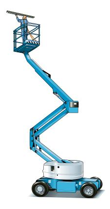
Figure 13 A mobile elevating work platform
